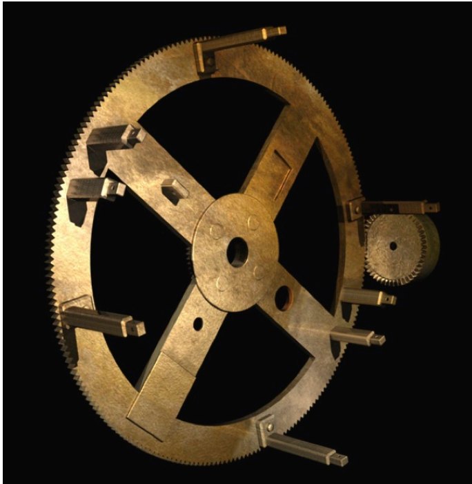
Fig.51: The eight pillars on the Main Drive Wheel (Freeth & Jones, 2012)
